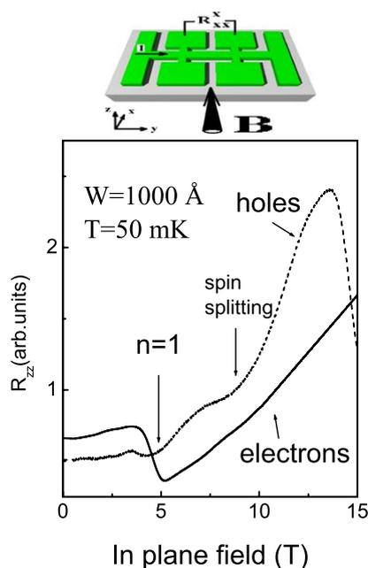
Fig. 4. Magnetoresistance of a 1000 Å PQW with 2D holes and electrons as a function of the in-plane magnetic field,  $T = 50$  mK. Current in hole PQW flows along  $[01\bar{1}]$  direction.
