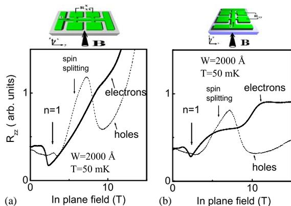
Fig. 5. Magnetoresistance of a 2000 Å PQW with 2D holes and electrons as a function of the in-plane magnetic field for the different experimental geometries: (a) in-plane component of the magnetic field is directed perpendicular to the current flow and (b) in-plane component of the magnetic field is directed parallel to the current flow. Current in hole PQW flows along  $[01\bar{1}]$  direction,  $T = 50$  mK.
