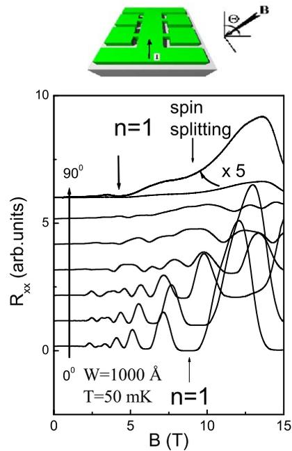
Fig. 2. Magnetoresistance of a 1000 Å PQW with 2D holes as a function of magnetic field for different tilt angle  $0^\circ < \Theta < 90^\circ$ ,  $T = 50$  mK. Arrows indicate the fundamental magnetic field  $B_1$  corresponding the depopulation of the last Landau level. Current flows along  $[0\ 1\ \bar{1}]$  direction.
