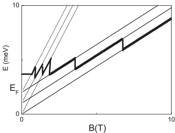
Fig. 3. Magnetic-field subband spectrum for three subbands and 2 LL. Thick line—Fermi energy.
