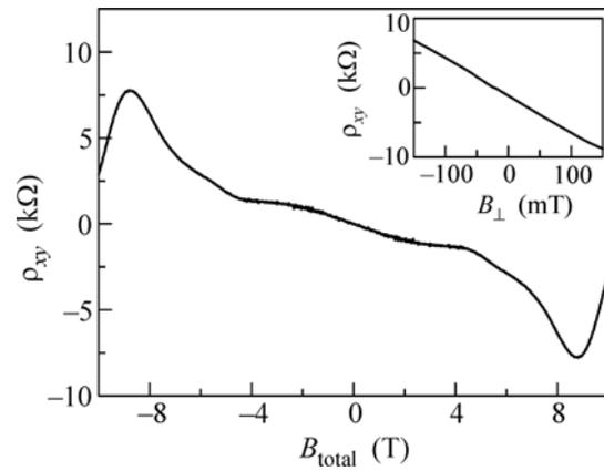
**Fig. 3.** Hall component of the resistivity versus the total magnetic field at the charge-neutrality point ( $N_s = P_s$ ) for  $T = 1.5$  K. Inset: the Hall resistivity at the charge-neutrality point versus the magnetic field with zero parallel component.
