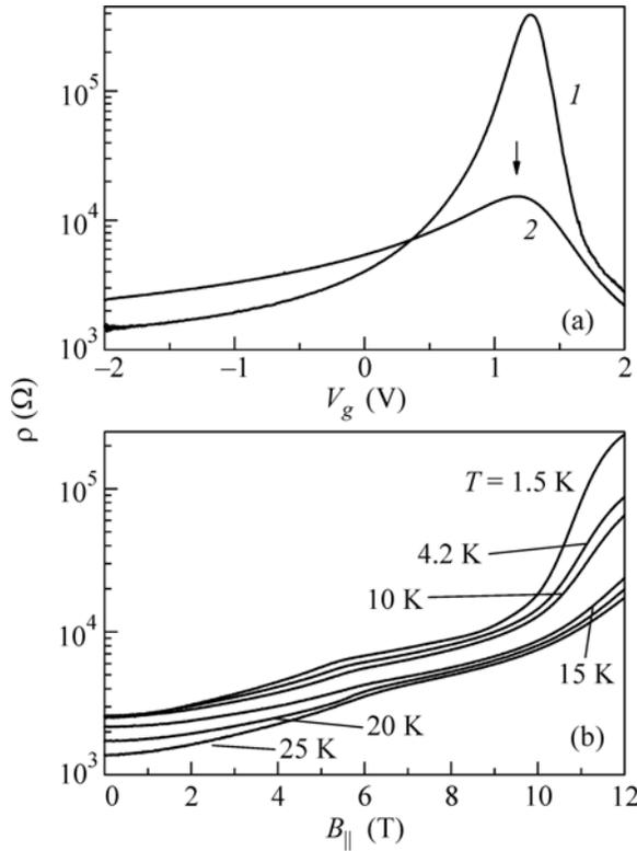
**Fig. 1.** (a) Dependences  $\rho_{xx}(V_g)$  for  $B_{||} = 12$  T and temperature  $T = (1)$  1.5 and  $(2)$  30 K. The arrow indicates the position of the curve peak, corresponding to the charge neutrality point ( $N_s = P_s$ ), which occurs at  $V_g = 1.173$  V. (b) Dependence  $\rho_{xx}(B_{||})$  for  $T = 25, 20, 15, 10, 4.2,$  and  $1.5$  K and  $V_g = 1.173$  V.
