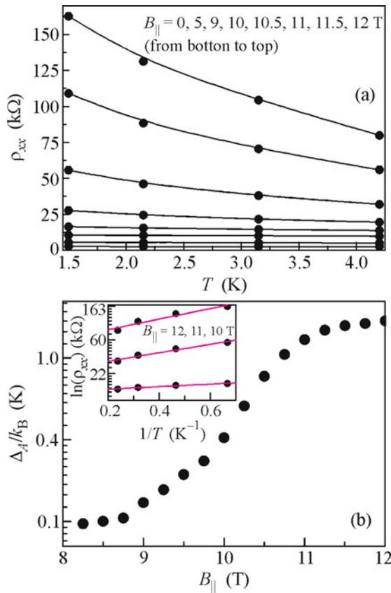
**Fig. 2.** (a) Temperature dependence of the resistivity in the range of 1.5–4.2 K for different values of the parallel magnetic field (lines are drawn through experimental points to guide the eye). (b) Energy gap  $\Delta$  at the charge-neutrality point ( $N_s = P_s$ ) for different values of the parallel magnetic field in the range of 8–12 T. Inset: approximation of the temperature dependences corresponding to parallel magnetic fields of 12, 11, and 10 T by Arrhenius curves.
