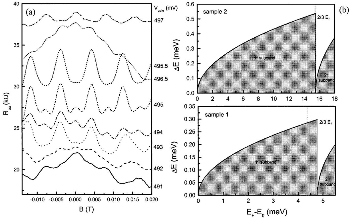
FIG. 3. (a) The variation of the AB oscillations with the gate voltage in symmetric ballistic ring uniformly covered by a gate; (b) dependence of the energy level spacing in the two samples versus  $(E_F - E_0)$ , where  $E_0$  is the bottom of the first subband, and  $E_F$  is constant, determined from experiment (the dashed line is the value of  $E_F - E_0$  used in our calculation).
