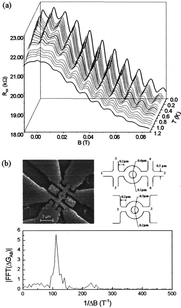
FIG. 1. (a) Set of magnetoresistance curves  $R_{xx}(B)$  for different temperatures, from 40 mK to 1.2 K; (b) Fourier transform of the 40 mK curve. Insert: Schematic view of the samples and microphotograph of the sample.
